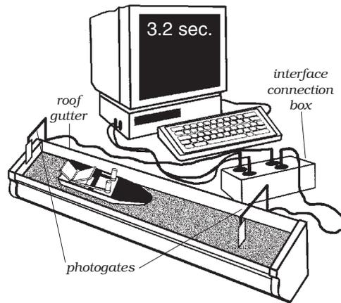
display it on the monitor. The boats must be equipped with a flag that will block the beam of light when the boat passes through the photogate. Photogates are available in kits or ready-made and range in price from a \$23 kit to \$75 assembled. Versions are adaptable to IBM, Apple II, and Macintosh computers; additional interface software will be needed. Available from:
